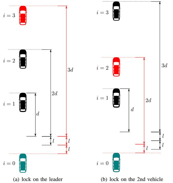
Fig. 5. Platooning strategy for host vehicle ( $i=0$ ). See text for explanations.
