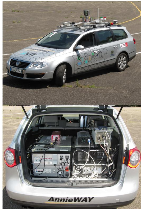
Fig. 2. The experimental vehicle (top) with its technical equipment in the trunk (bottom). The bottom image shows the power supply on the left, the GPS/INS unit on top (red box), and the control computers on the right.
