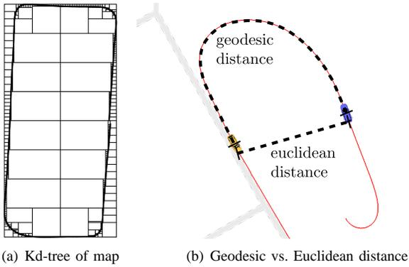
Fig. 4. Our maps are stored in kd-trees, as shown in (a) for one of our testing grounds. This allows for fast map matching and evaluation of geodesic distances between vehicles on the same lane (b).
