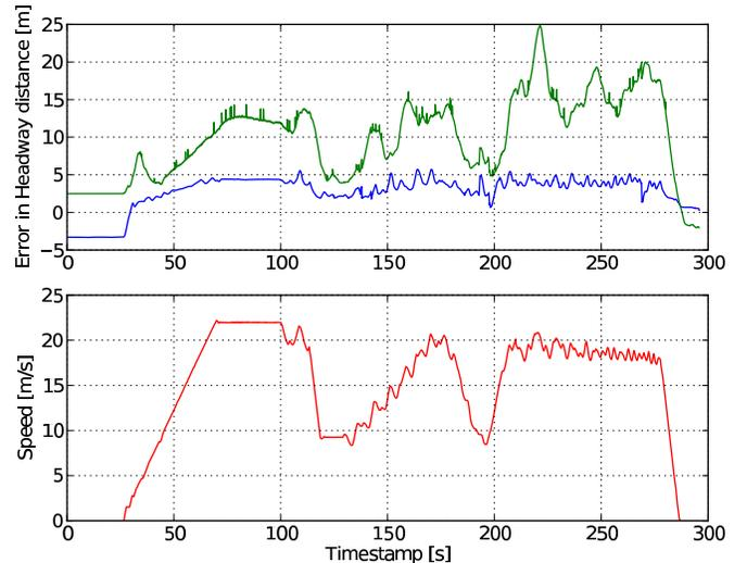
Fig. 7. The top plot shows desired headway distance minus real headway distance for AnnieWAY (blue) and Halmstad (green) in a run where both were directly behind the lead vehicle. The bottom plot shows the speed profile of the lead vehicle in the same run.
