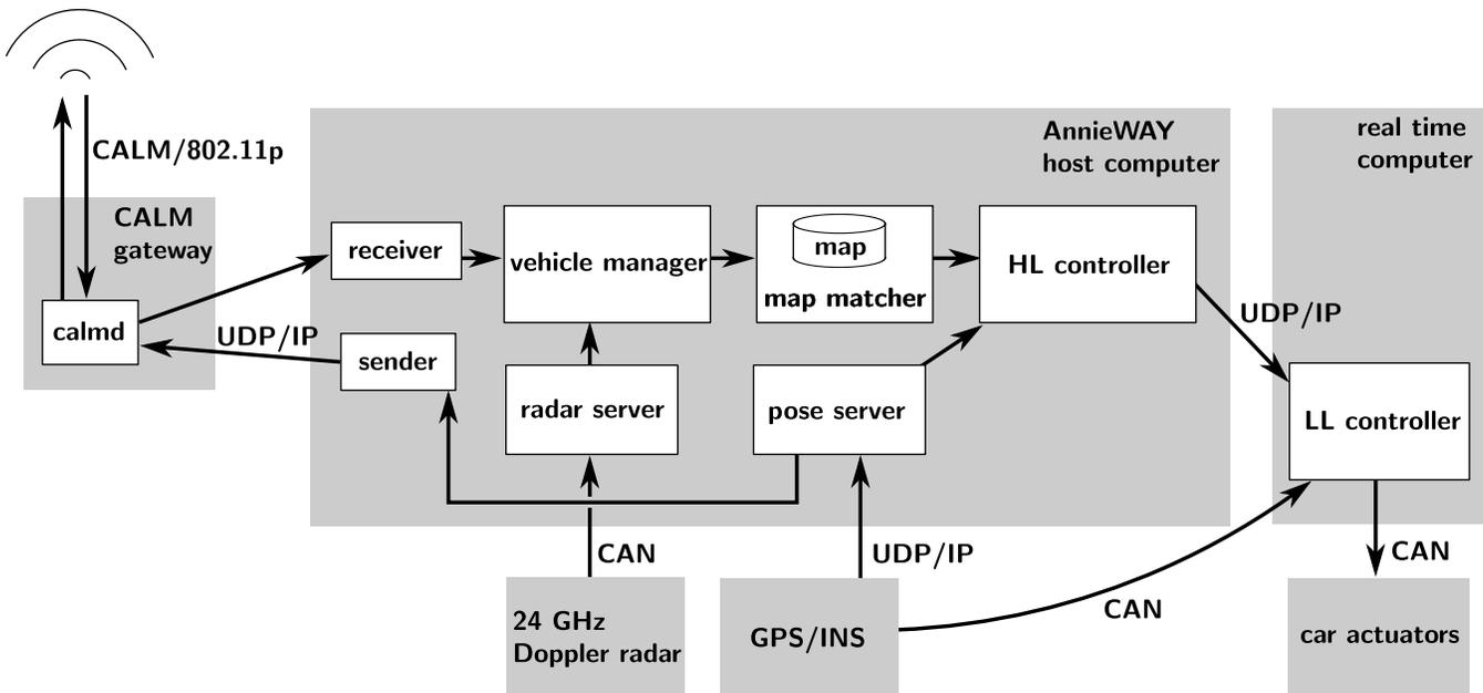
Fig. 3. GCDC system architecture. See Sec. II for explanation.
